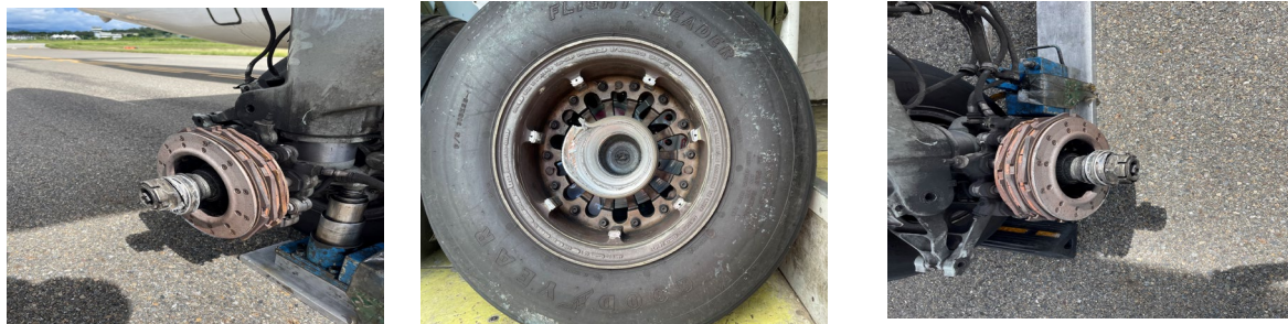
Figure 1- RH outboard Mainwheel detaches from P2-ANO aircraft on landing roll.
