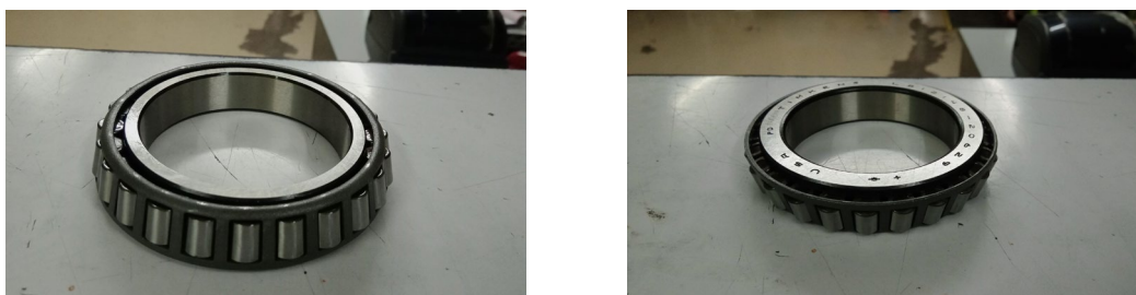
Figure 2- New main wheel bearing cone assembly showing rollers located in the cage
