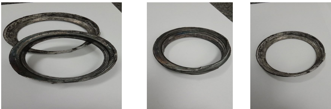
Figure 5 – damaged mainwheel bearings and its cup
