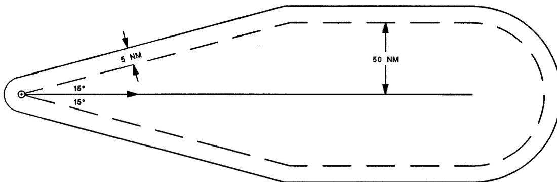
**Example 9 :** As for example 2, but  $12^\circ$  lines expand to maximum distance of 50 NM either side of track. In no case is the maximum width, inside the 5 NM buffer area greater than 50 NM either side of track.
