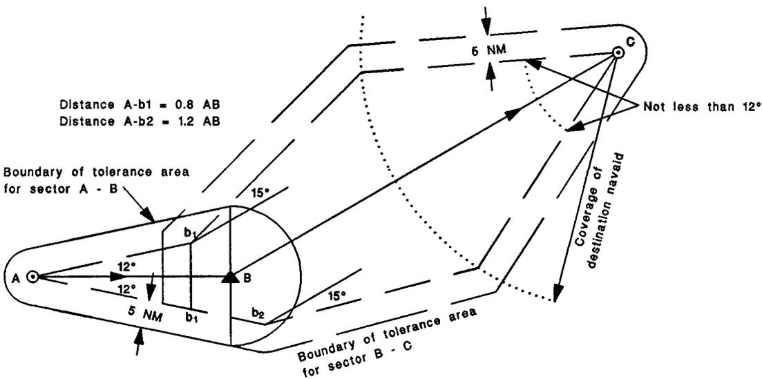
**Example 13 :** Route segment with change of direction at DME/Azimuth aid fix. Coverage of destination navaid not less than length of second sector of route segment. NB Diagram shows DME at A – the DME fix area would be different if DME is in a different position.
