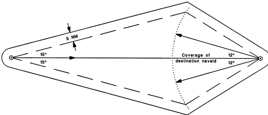
**Example 5 :** Navaid at departure end but not at destination, with segment distance not exceeding 235 NM (12° diverges 50 NM from track in 235 NM). This example assumes a minimum rated coverage of at least 235 NM.
