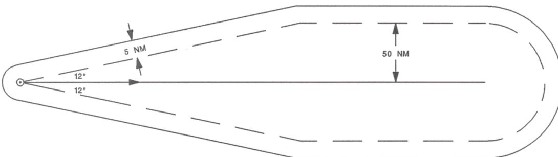
**Example 7 :** Route segment without nav aids, with segment distance not exceeding 186 NM ( $15^\circ$  diverges 50 NM from track in 186 NM).
