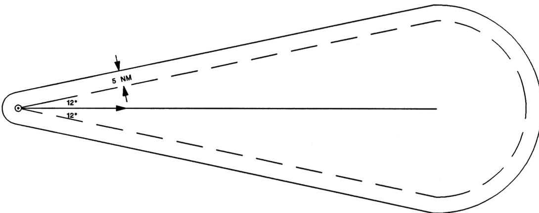
**Example 6 :** Navaid at departure end but not at destination, with segment distance exceeding 235 NM.
