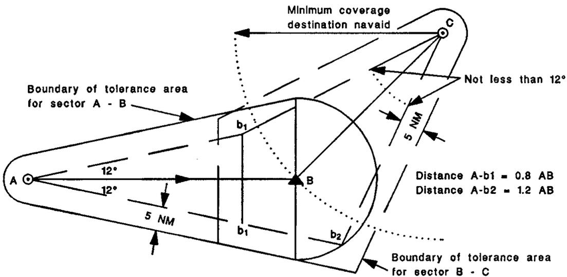
**Example 12 :** Route segment with change of direction at DR position. Coverage of destination navaid less than length of second sector of route segment.
