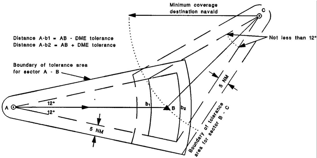
**Example 14 :** Route segment with change of direction at DME/Azimuth aid fix. Coverage of destination navaid less than length of second sector of route segment. NB Diagram shows DME at A – the DME fix area would be different if DME is in a different position.
