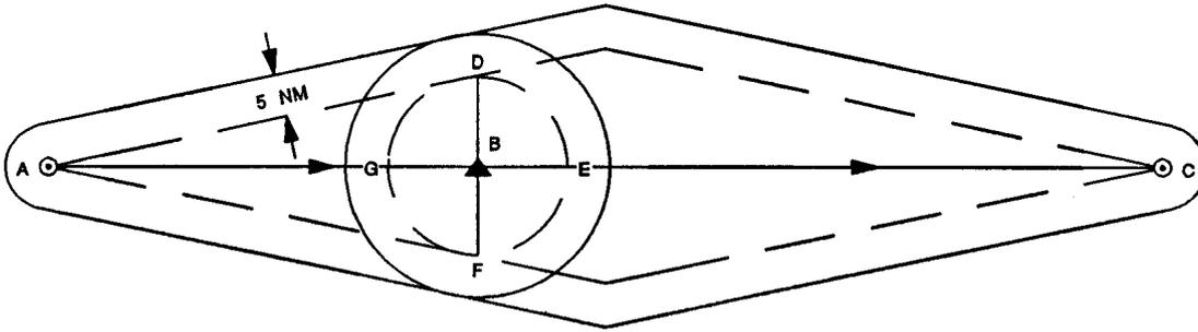
**Example 11 :** Route segment with change of direction at DR position. Coverage of destination navaid not less than length of second sector of route segment.
