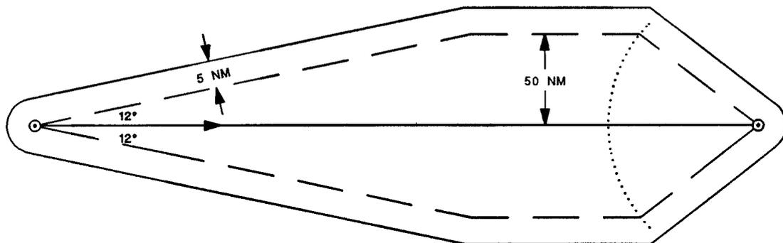
**Example 10 :** Route segment with intermediate reporting point (no position fix). The basic area for A – B is ADEF and, for B – C, is GDCF.
