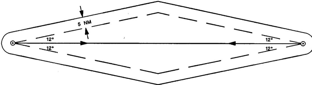
**Example 2 :** Route segment with navaids at each end, where coverage from the destination navaid is less than half the segment length, but navaid at departure end covers the distance up to at least the coverage of the destination navaid.
