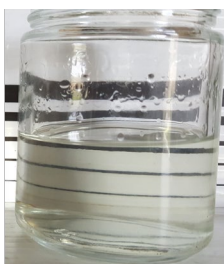
Figure 1- Pictures of Aviation fuel contaminated with dissolved water, dispersed and free water
