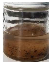
Figure 1- Pictures of Aviation fuel contaminated with dissolved water, dispersed and free water
