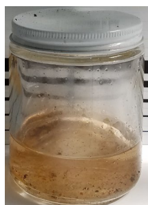
Figure 1- Pictures of Aviation fuel contaminated with dissolved water, dispersed and free water
